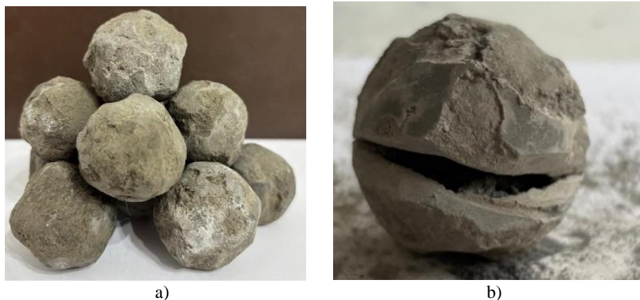
Fig.1. Non-kilned ash-slag gravels: a) – single component structure; b) two component structure.
