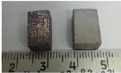
Fig.7. Samples D16_(N+X) and D16_(N+X)_U12 after exposure to the test solution for the control time: on the left is sample D16_(N+X); on the right is sample D16_(N+X)_U12.
