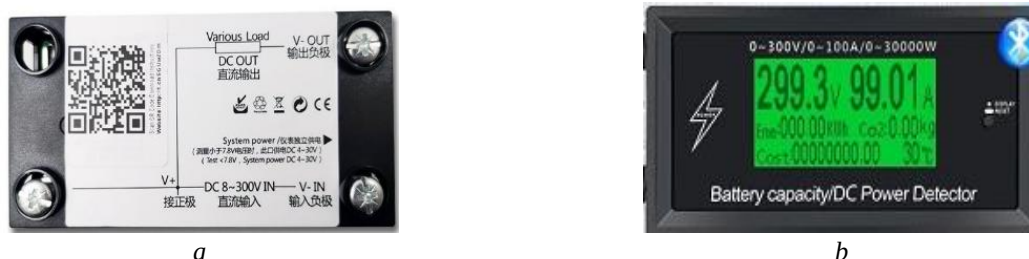
Fig. 5. ATORCH DT3010 wattmeter: (a) front view; (b) rear view with connection diagram
