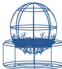
Fig.4. The contact field of the ball-seat valve pair elements
