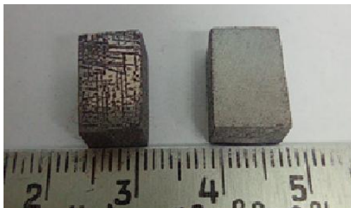
Fig.7. Samples D16_(N+X) and D16_(N+X)_U12 after exposure to the test solution for the control time: on the left is sample D16_(N+X); on the right is sample D16_(N+X)_U12.
