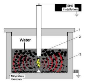
**Fig.1.**Working area for processing oil bottom sediment by electrohydroimpulse discharges: 1-cover; 2-positive electrode; 3-negative electrode
