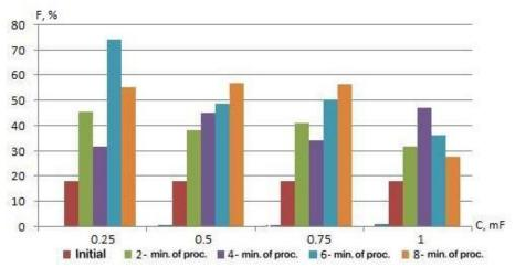
**Fig.3.**Influence of the capacity of the switching device on the increase in the yield of light and medium fractions from the OBS of the reservoirs of the Atasu-Alashankou station at the different interelectrode space
