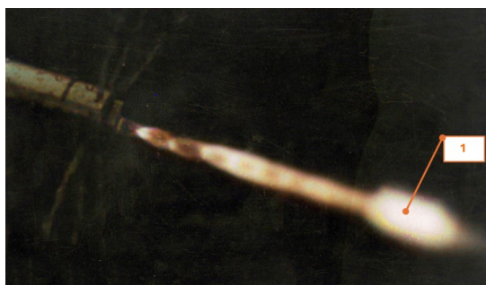
Fig.4. Jet outflow from the nozzle of a thermal tool (see Fig. 1) for spraying: 1 – strong flame swelling due to spin detonation of a supersonic high-temperature jet.
