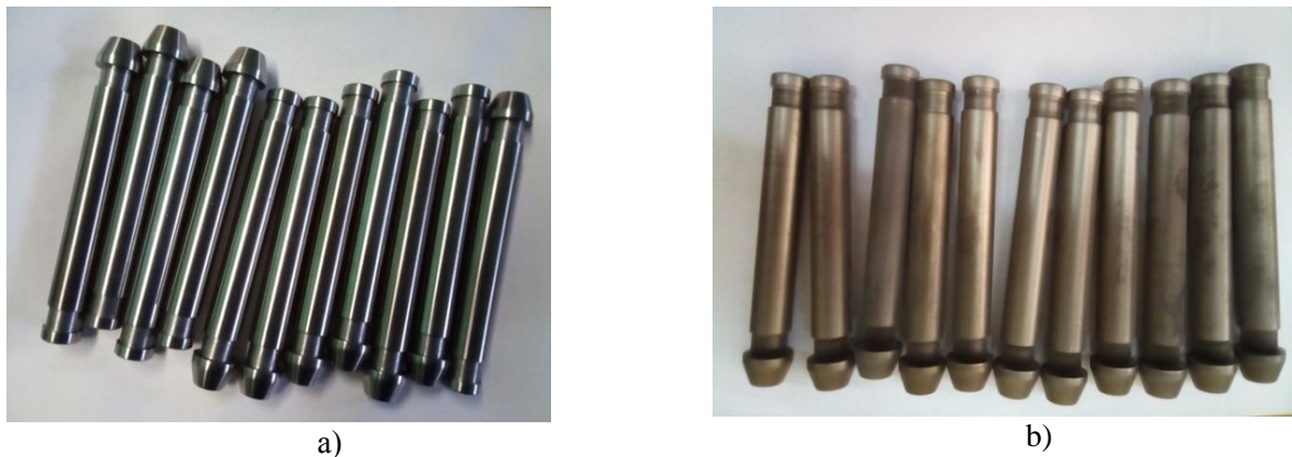
Fig.3. Stocks 35HGSA before (260 HV) (a) and after (820 HV) (b) nitriding
