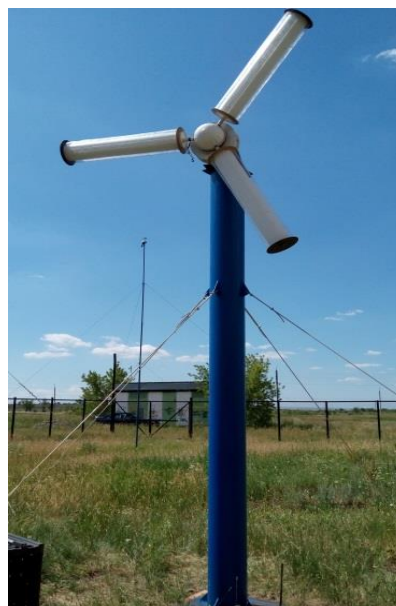
Fig.2. General view of an experimental model of WPP with cylindric blades
