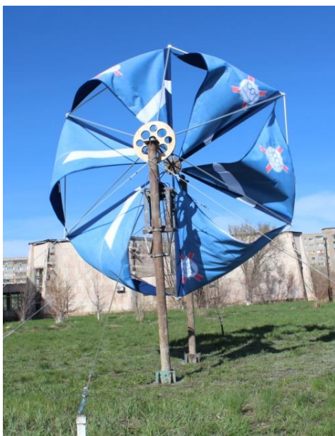
Fig.1. General view of an experimental sail-type WPP model
