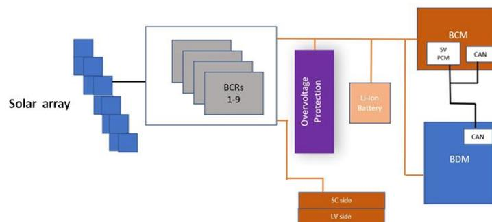
**Fig.2.** Electrical architecture of the KazEOSat – 2.
