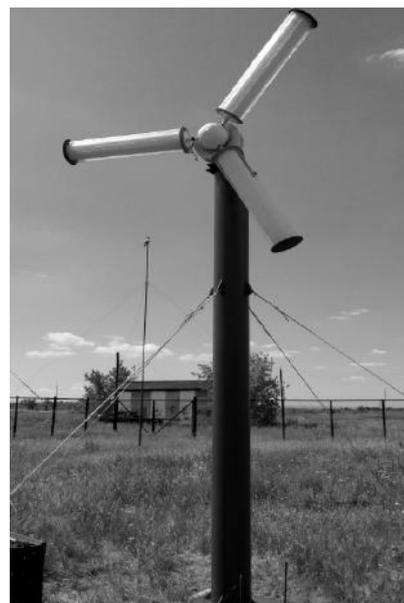
Fig.2. General view of an experimental model of WPP with cylindric blades
