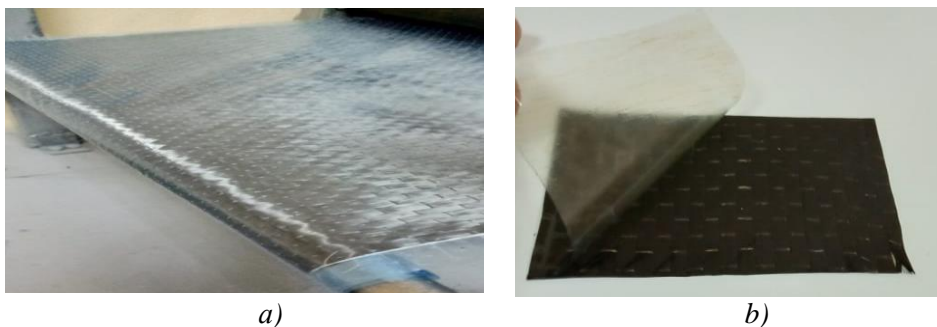
Fig.2. Roll of experimental prepreg sample (a), experimental prepreg sample (b)
