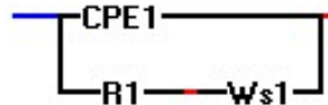
Fig.3. Equivalent electrical circuit, where R_1 is active resistance; CPE - constant phase element; W_{s1} is the “final” Warburg element characterizing the diffusion properties of the sample.
