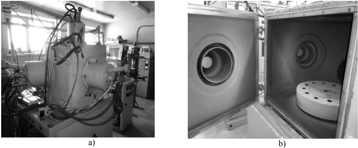
Fig. 2. Vacuum chamber of the NNV 6.6-11 installation (a) and the satellite of the rotating table (b)
