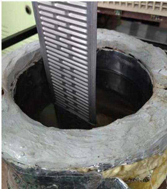
**Fig. 2.** General look of a crystallizer tank with a plate
