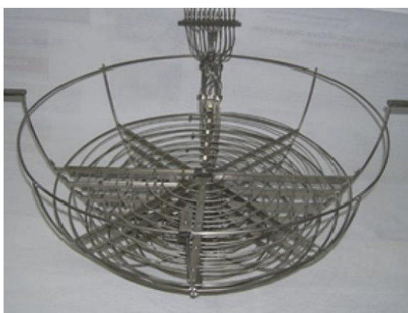
Fig. 6. Ohmic heater in LIVE experiment
