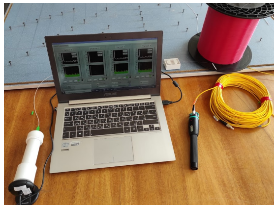
Fig. 2. Laboratory sample of a fiber optic sensor based on a Mach-Zehnder interferometer
