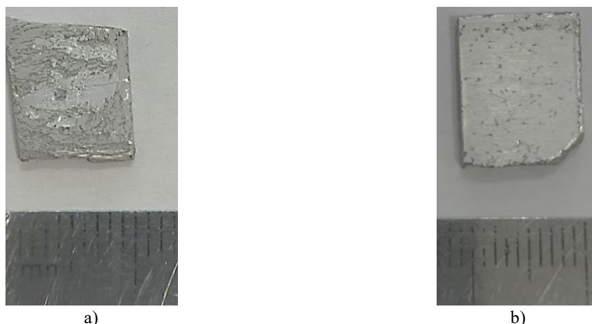
Fig.4. Photographs of the surface of samples exposed to alcohol solution of iodine for 72 hours: a) an untreated AMg2 sample; b) a sample treated with ozone for 6 hours.
