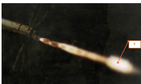
Fig.4. Jet outflow from the nozzle of a thermal tool (see Fig. 1) for spraying: 1 – strong flame swelling due to spin detonation of a supersonic high-temperature jet.
