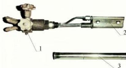
Fig.1. Unit for 1 an automated line. The combustion chamber is cooled by coatings 2 (granite); 3 – housing.
