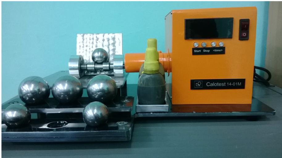
**Fig.5.** A device developed by us for testing materials and coatings for microabrasive wear
