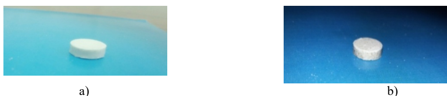
Fig.2. Modified PTFE samples obtained a) cold pressing, sintering at the temperature T = 393^{\circ}\text{C} and rapid quenching; b) after sintering at the temperature T = 393^{\circ}\text{C} , slow quenching and standing under the press for a day.
