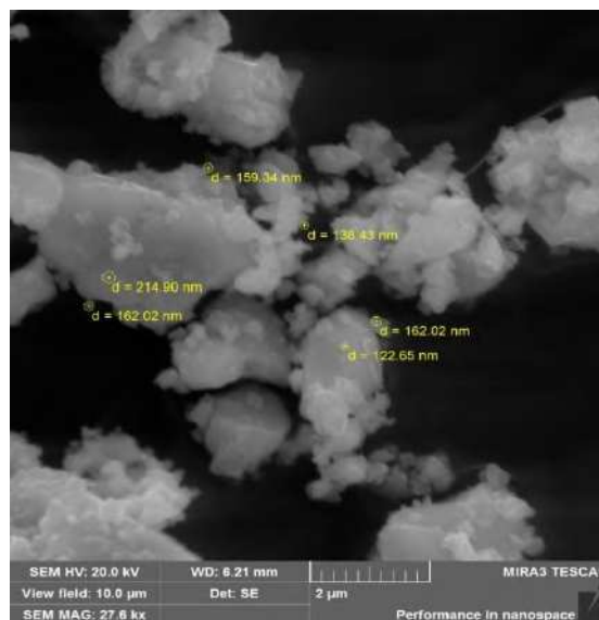
Fig. 1. The electron microscopy of the nanostructured \text{LaMgCuZnMnO}_6
